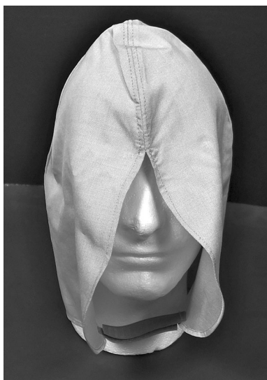
Fig. 6 A photograph of a sleeping cap sewn from the microwave-shielding fabric
